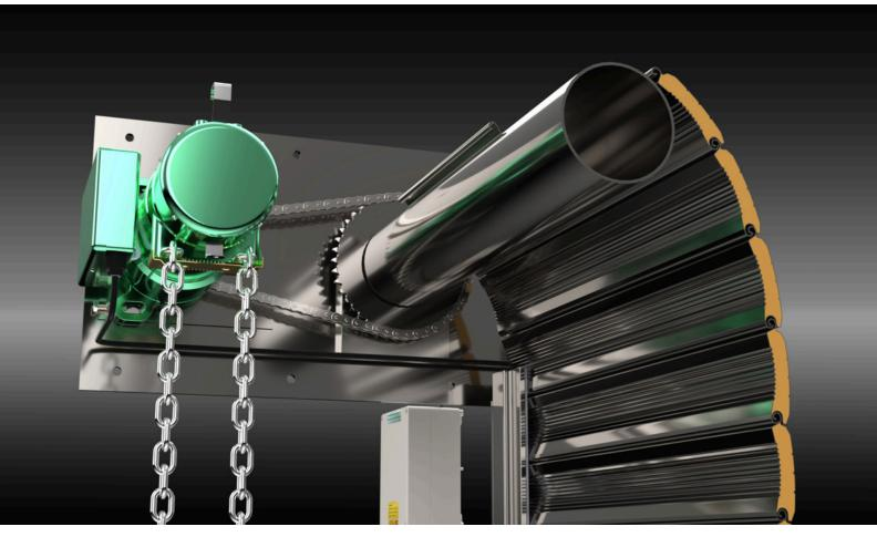
**Shutter Curtain:** Manufactured using 95mm insulated galvanised or plastisol material. The 95mm foam-filled lath features a dou- ble-skin profile, roll-formed from a single steel coil. Its Thermal performanace is 3.3W (m2k), its has an acoustic rating of 22db and is category 5 wind tested.
