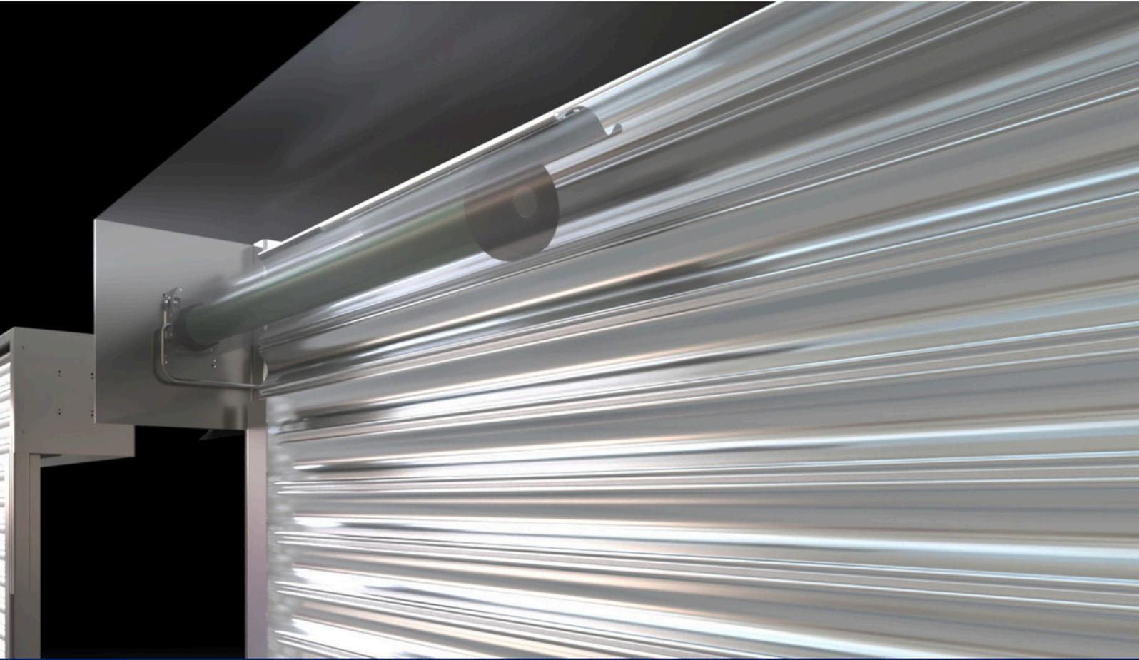
**Shutter Curtain:** Manufactured using 3" (75mm) galvanised or plastisol lath, with the gauge (22g, 20g, 18g) of lath selected based on the specific application size. The laths are secured with endlocks, which can be made of steel, plastisol, or cast material, depending on the requirements, to ensure the curtain remains properly positioned within the guides.
